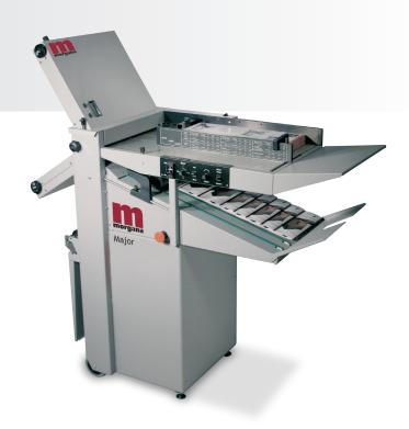
The plug-in perforator/scorer is a standard feature of the Morgana Major and work is delivered into a catch tray. The plug-in unit can be used to act as a roller bypass facility, allowing cover stock to be folded and delivered flat.
